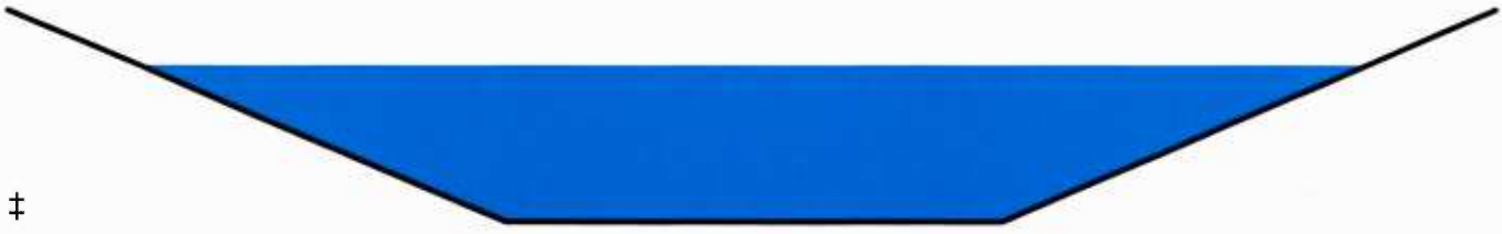
Reach 5R: GRASS SWALE TO CONC CHAN
